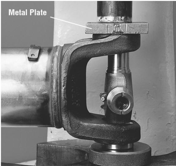
5. Place a push rod that is smaller than the diameter of the bearing cup assembly under the bearing cup assembly and continue pressing into the yoke cross hole until far enough to install a snap ring.
