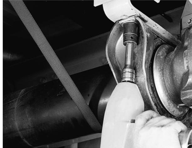
4. Using a puller, follow the tool manufacturer's instructions to remove the yoke and center bearing companion flange. Both the yoke and companion flange are press fit and should **NOT** be removed with a hammer. If either the yoke or companion flange are loose enough to be removed by hand, the entire coupling shaft must be replaced. Remove and discard slinger from the yoke.
