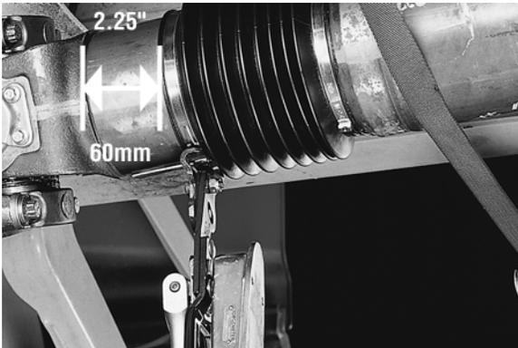
4. Position a clamp on each end of the new boot. Slide the boot onto the grease-free yoke shaft shoulder.
