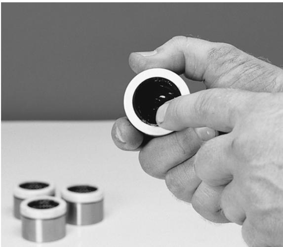
**Caution** - Spicer **DOES NOT** recommend wiping the outside of bearing cup assemblies or yoke cross holes with grease, oil or silicone-based sprays. This could result in bearing cup assembly rotation in yokes.
