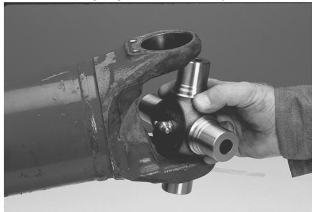
**Note:** Always inspect bearing cups for rollers that may have fallen (downed rollers) out of place before installation.
