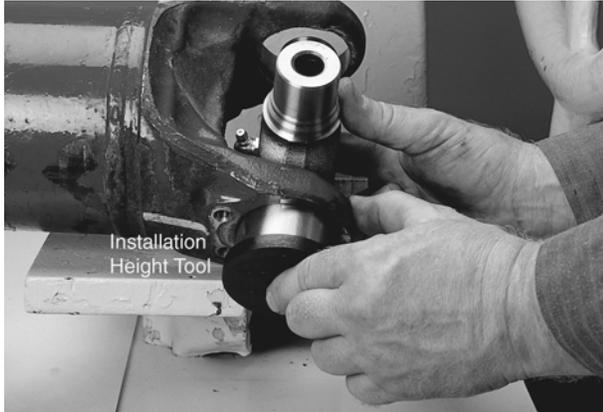
4. Align the yoke in an arbor press with the bearing assembly resting on the base of the press. Cover the yoke ear with a metal plate that has 0.25 inch (6.4 mm) minimum thickness. Push the yoke onto the bearing cup assembly until it is flush with the cross hole face. **Do not remove the installation height tool.**
