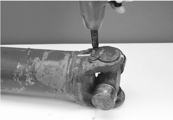
2. Make sure universal joints cross assembly is not tilted in the yoke. Place bearing cup spacer onto the base of the arbor press and under the yoke. If the arbor is larger than the bearing cup diameter, a smaller diameter push rod will be needed to avoid damaging the yoke or bearing.
