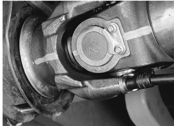
5. Working at the effected universal joint, support the driveshaft with a support strap. Attach support straps to frame rails or some structural part of the vehicle.
