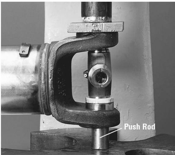
6. Remove yoke from arbor press. Install a snap ring using snap ring pliers.
