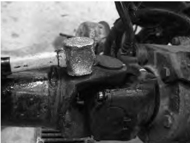
2. Apply grease gun pressure and purge all four bearings until fresh grease is seen at all four bearing seals.
