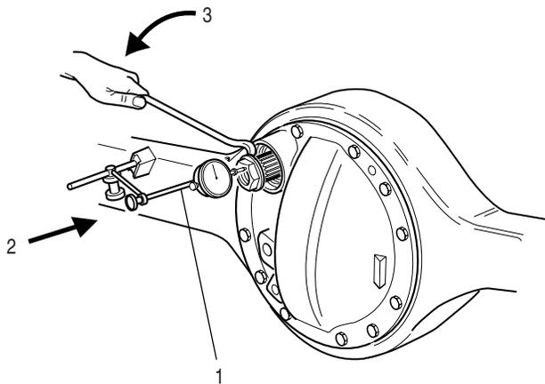
**Note:** The output yoke can be installed when taking end-play measurements.
