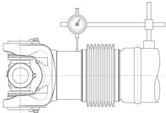
2. Arrange dial indicator with magnetic base one-quarter inch (1/4") from the driveshaft's tube weld. Dial indicator should be firmly mounted on the tube so that **no** movement of the dial indicator base is allowed.
