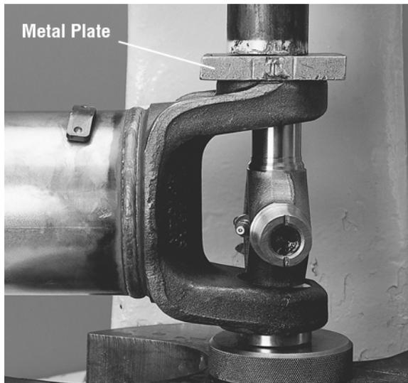
5. Flip yoke 180 degrees. Position the remaining installation height tool on the end of another bearing cup assembly. Place bearing cup assembly over trunnion diameter and align it to the yoke cross hole. Push the bearing cup assembly until both installation height tools are flush with the cross hole face.
