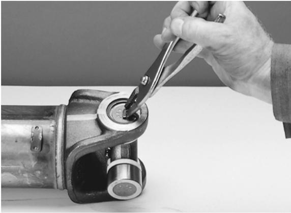
1. **For Quick Disconnect™ Style:** Remove spring tab bolts and discard, and remove outboard bearing cap assemblies.
