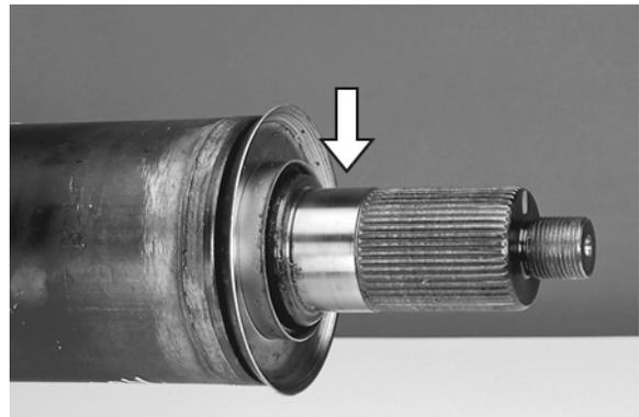
6. If no damage is apparent, remove slinger and discard. Proceed to installation of center bearing.
