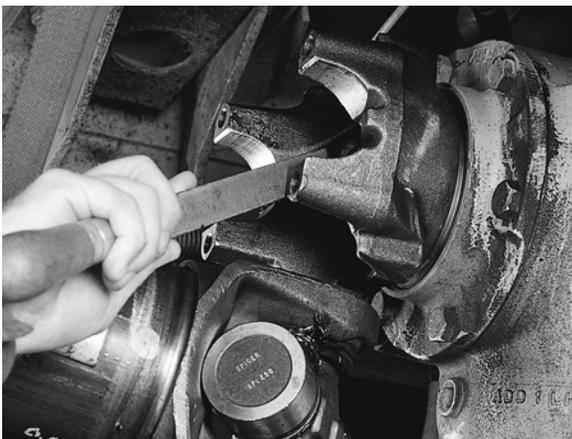
8. Inspect the end yoke cross holes for distortion and damage.
