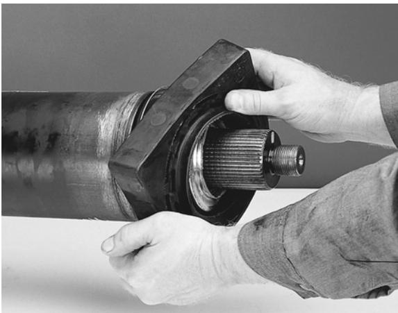
4. Using a puller, follow the tool manufacturer's instructions to remove the bearing assembly from the midship. Discard the center bearing.
