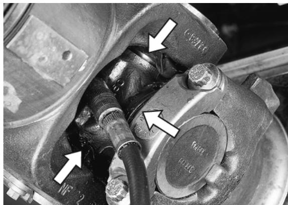
2. If any of the seals fail to purge, try to push the trunnion away from the bearing cup while applying grease. On two side zerk fittings, try greasing from the opposite side of the fitting.
