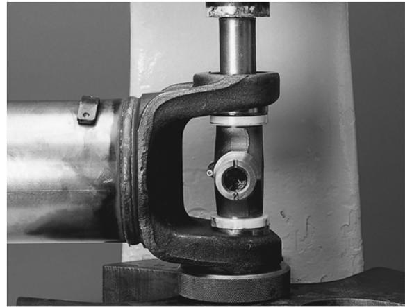
8. Remove yoke from arbor press. Install a snap ring using snap ring pliers.
