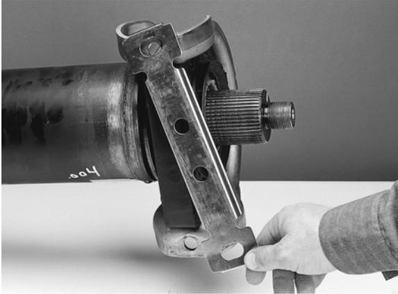
2. Remove and discard the center bearing bracket.
