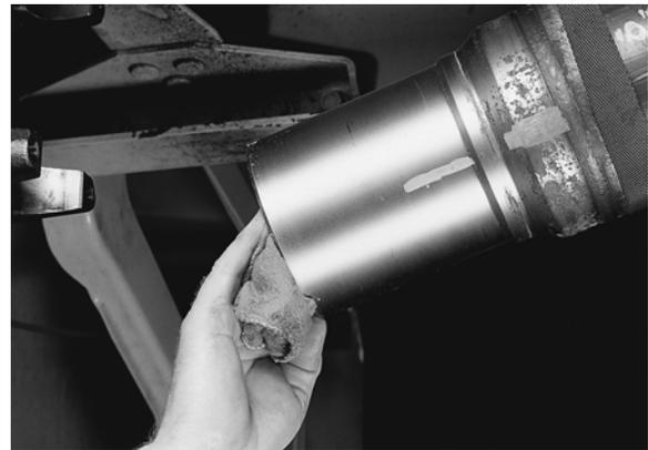
2. After all traces of grease and cutting solvent have been removed from the yoke shaft and spline sleeve, apply half of the grease provided to the yoke shaft splines and the other half to the spline sleeve, cover the entire splined surface.
