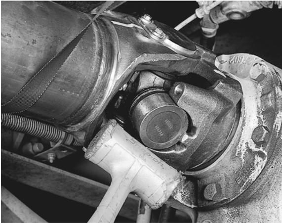
5. Remove bearing retainers or stamped straps and bolts at the **front** end.
