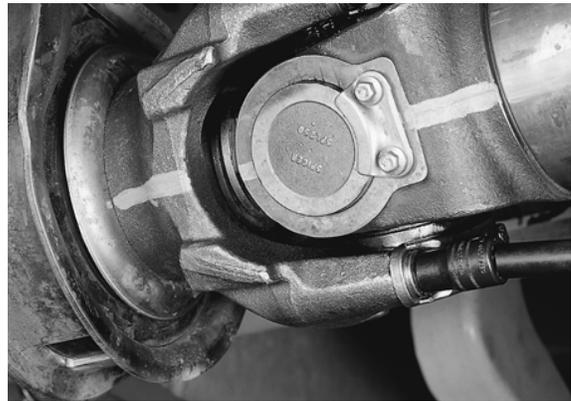
3. Align the bearing cups with the yoke ears making sure that the cups are evenly spaced between the nibs of the yoke. A soft faced hammer can be used to fully seat the bearing cups into the yoke.
