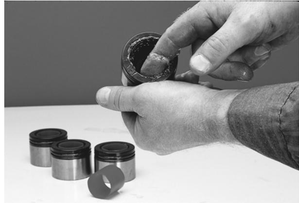
**Caution - Spicer DOES NOT** recommend wiping the outside of bearing cup assemblies or yoke cross holes with grease, oil or silicone-based sprays. This could result in bearing cup assembly rotation in yokes.
