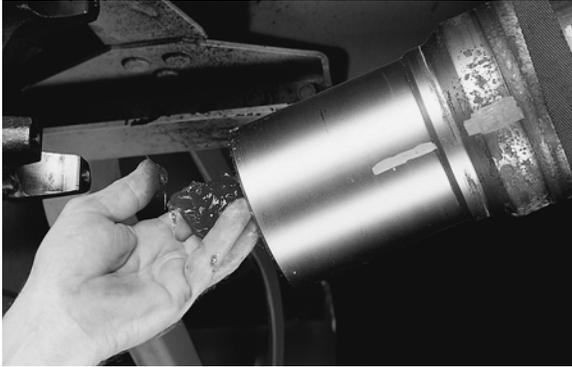
3. Measure and place a mark 2.25 inches (55-60mm) from yoke shaft shoulder with a marking stick, paint marker or other legible marking device.
